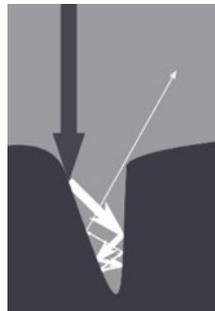
Figure 5: Schematic of the electron backscattering influenced by a pore. [3, 4]
